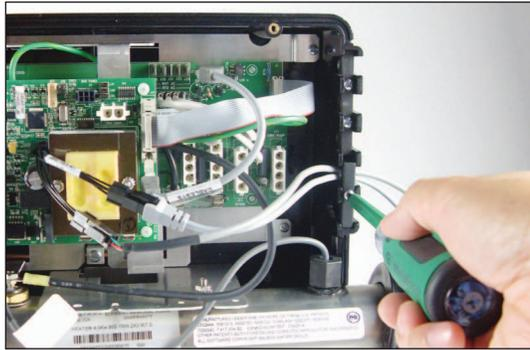
– Insert the plastic holder and screw back in place. Make sure the 2 cable wires are secure in place.
