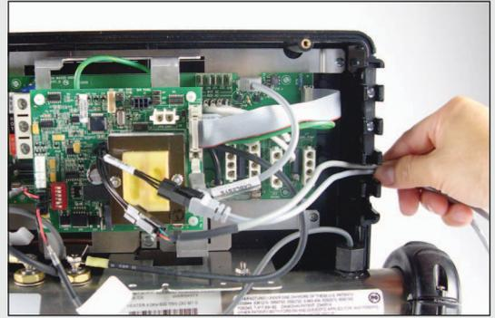
– Place the Wi-Fi cable and Control Panel cable inside the wire holder.
