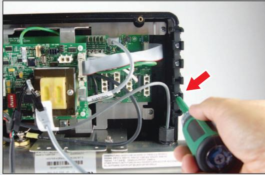
– Remove 1 screw to open the cable holder.
